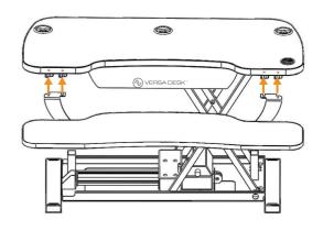
Make sure the keyboard tray is all the way in and the end of the keyboard tray is sitting under the middle bracket.
