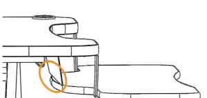
Secure the side brackets to the top surface by fully tightening all 4 thumb screws.
